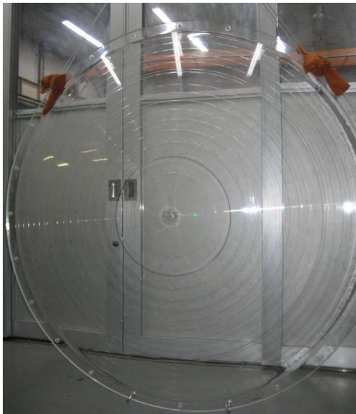
Acrlic \phi 1.5\text{m} Large fresnel lens Riken Corp
