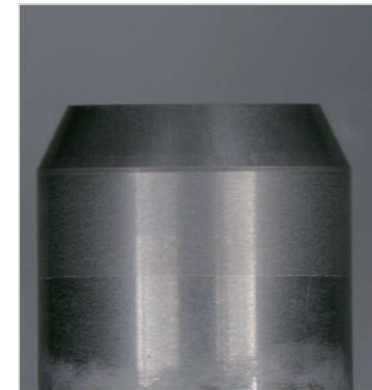
PCD (poly crystal diamond) micro rotating tools
