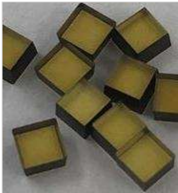
Single crystal diamond used for cutting edge
